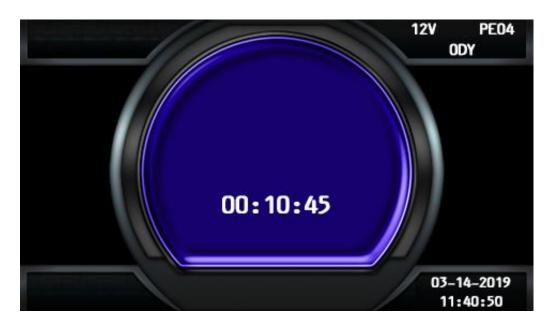
Charging starts after the programmed delay. The charger uses Profile, Capacity and Temperature settings programmed in the Configuration menu.
