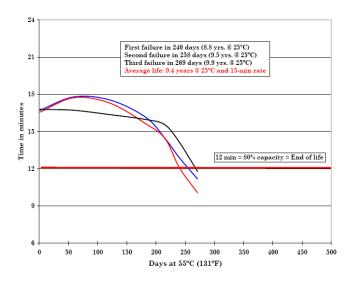
Genset starting batteries typically stay on continuous float or trickle charge for months or even years, and must be available to deliver the same cranking capability over its life. The TPPL battery is designed to last many years at room temperature when placed on continuous float charge and test data shown in the graph
