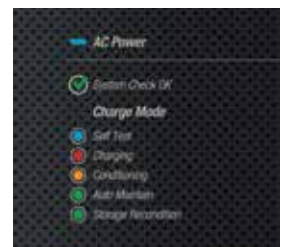
Charge Mode Status Indicator identifies each stage of charging
