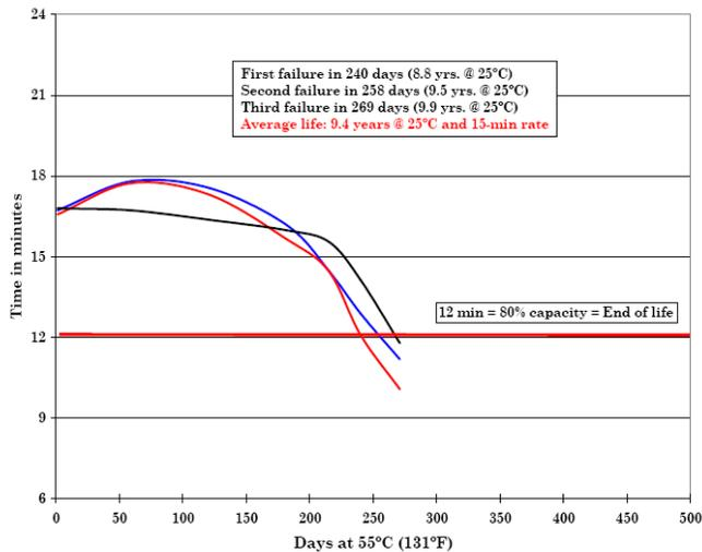
Genset starting batteries typically stay on continuous float or trickle charge for months or even years, and must be available to deliver the same cranking capability over its life. The TPPL battery is designed to last many years at room temperature when placed on continuous float charge and test data shown in the graph
